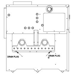
Figure 3 – Draining Pool Heater
